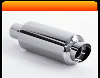
DTM-140 4.5" ROUND W/ 3" SLANTED ID 02.25" BL 11.00" BH 04.50" OD 03.00" BW 04.50" OL 15.25"
