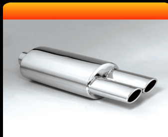
DTM-138 OVAL W/ DUAL OVAL ROUND SLANTED ID 02.25" BL 14.00" BH 05.00" OD 08.00" x 02.25" BW 08.00" OL 24.50"
